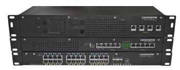
Yacht Router in combination with Network Expander Pro and Mobile Expander Pro as complete network solution for larger vessels.
